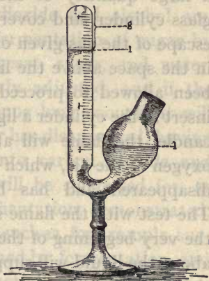
FIG. 66.—Fermentation-tube. l , level of fermenting liquid; g , space filled with gas ( \text{CO}_2 ) given off by fermentation.
